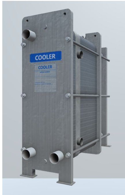
Figure 3 Plate Cooler (Unity View)
